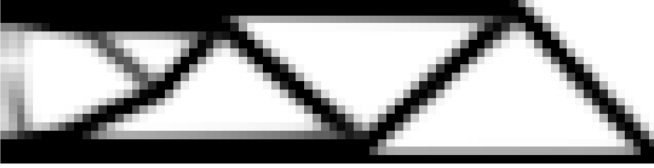
Fig. 2: Initial topology optimization results from Table I [2], [3].
