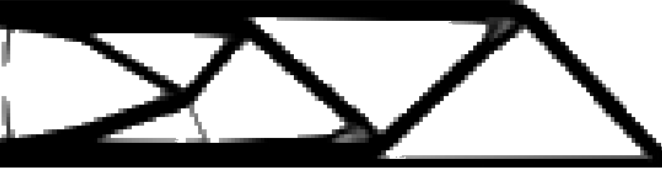
Fig. 3: Example of fine mesh topology optimization results from Table I, which was not favorable over coarser meshes [2], [3].
